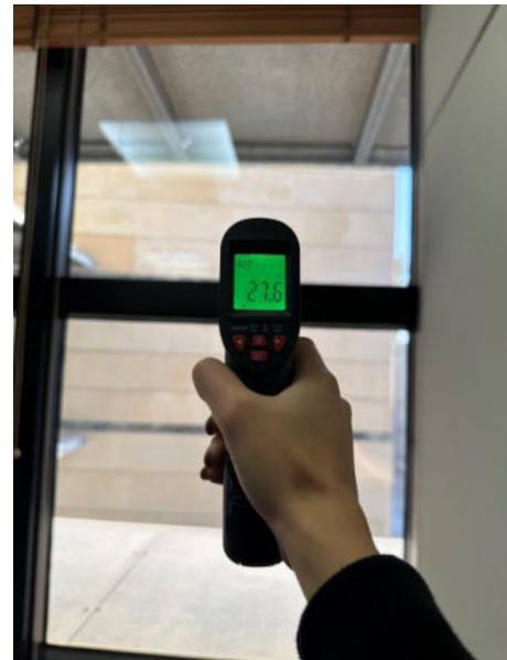
Figure 30: Northwest office window frame at 14:00, 27.6 °C
