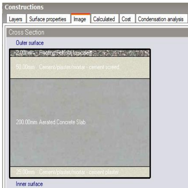
Image 5.6.6a: Roof construction
